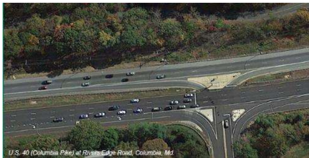
Figure 14: Example of a Continuous Green T-Intersection
