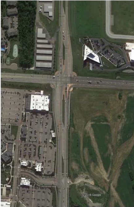
Figure 15: Examples of Displaced Left Turns in Ohio and Utah
