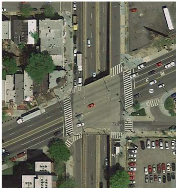
Figure 16: Examples of Compressed Diamond Interchanges in the District of Columbia and in Virginia
