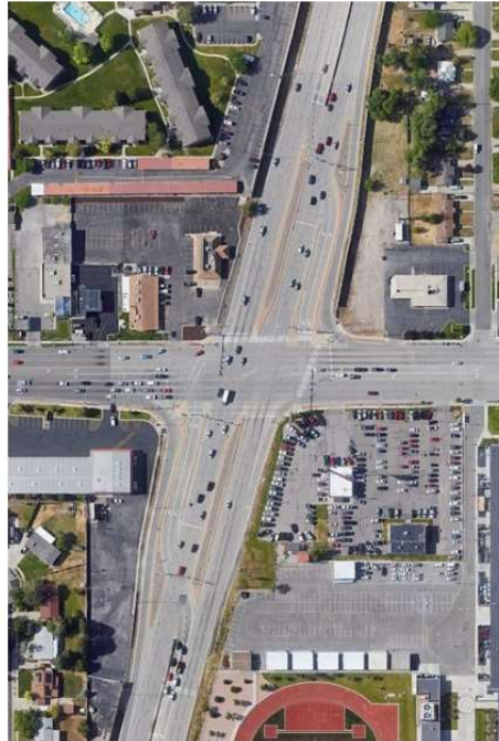
Figure 15: Examples of Displaced Left Turns in Ohio and Utah
